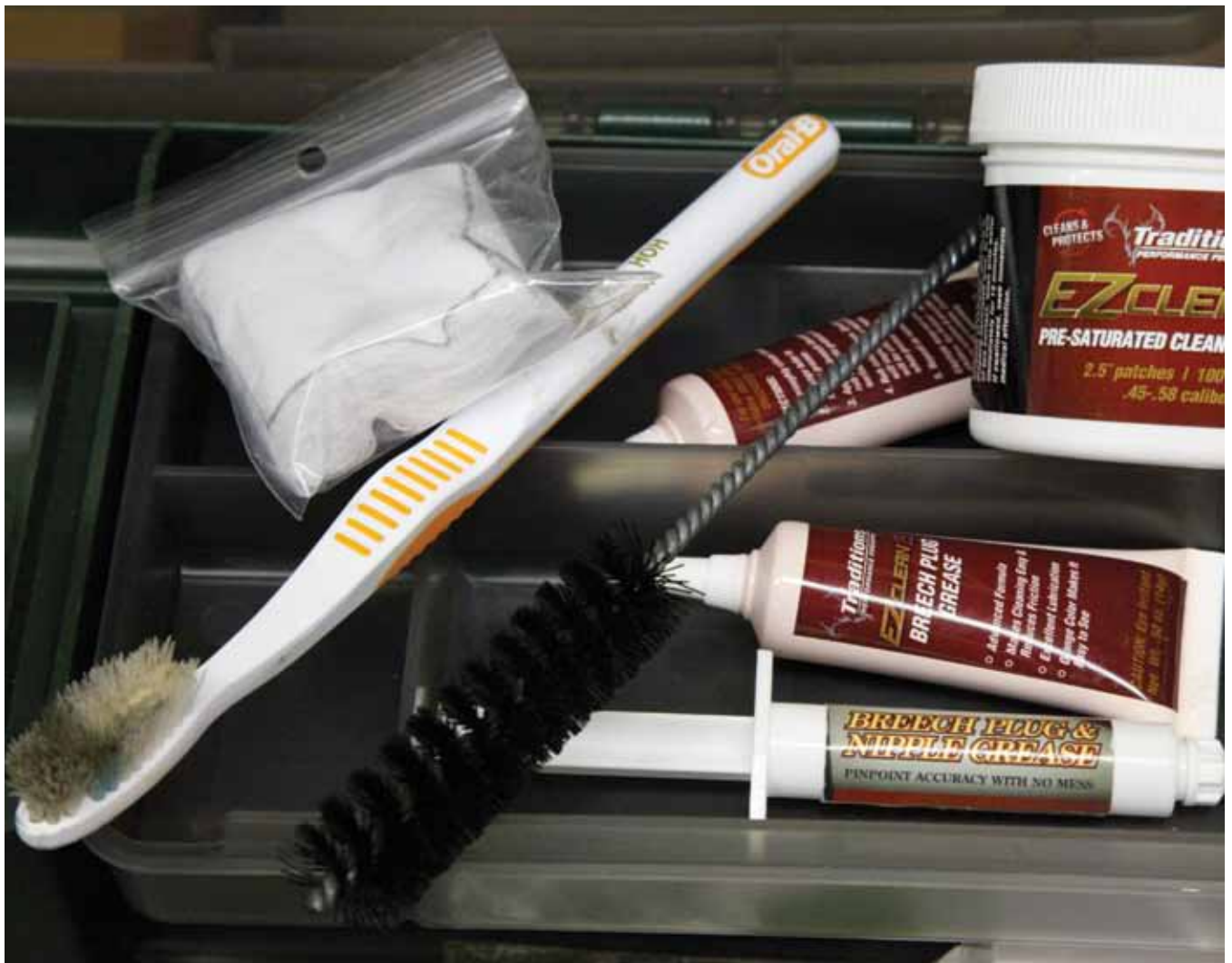
There are separate brushes sold for the breech threads, which allows you to use a short wire handle to twist and clean them properly, but old toothbrushes also work well.
