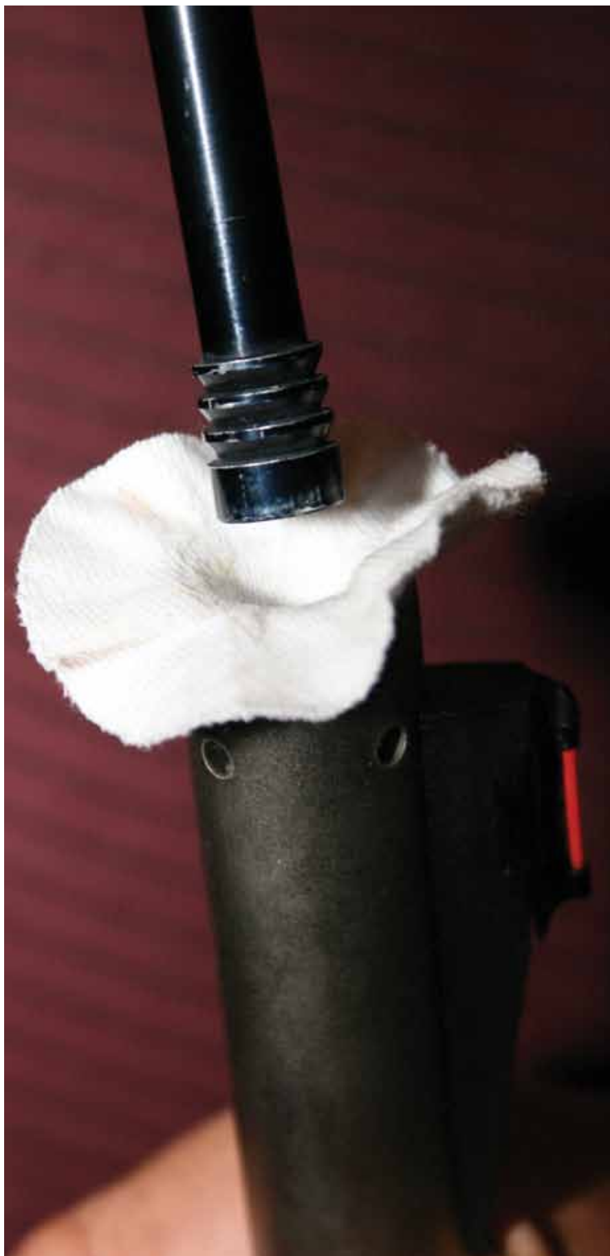
Once your pre-soaked patches start exiting the barrel without showing black fouling you can begin pushing dry patches.
