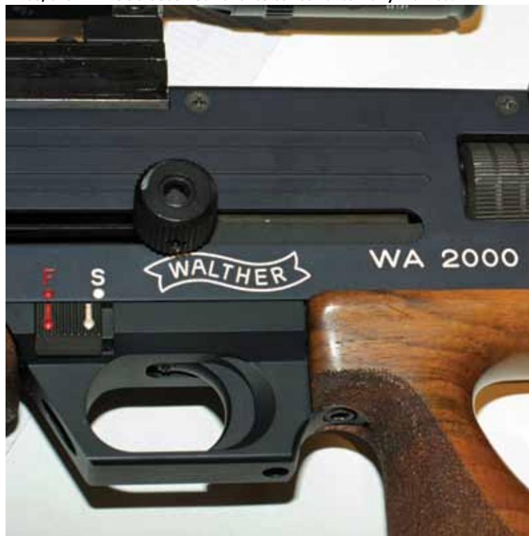
A close up of the safety, charging handle and barrel nut. Unlike most rifles, the WA-2000 does not have its caliber externally marked.
