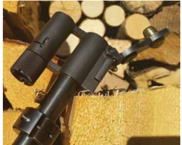
Megan's front sight is unusual and was one of only two such modifications on the World Cup circuit last season. The front sight cover springs have been removed and a small copper weight added, which causes the sights to open and close when she gets into or out of shooting position.
