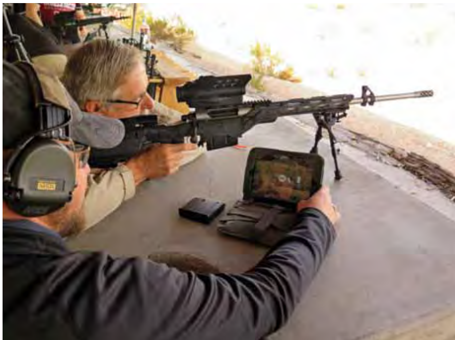
Tracking Point Rifles feature a high-tech blend of rifle and scope, including allowing a spotter with a tablet the same view as the shooter. They are reportedly banned from export, even to Canada.
