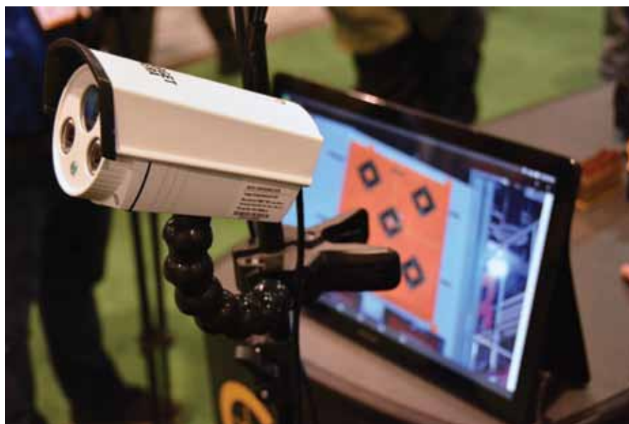
Affordable target systems, like this Caldwell model, use a camera mounted near the target. They send an image of the paper target back to the firing line, where it's displayed on a tablet or smart phone.
