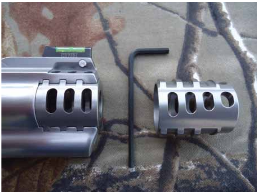
The muzzle breaks can be changed in a couple of minutes to suit the loads you are shooting and reduce the muzzle climb to a controllable push.
