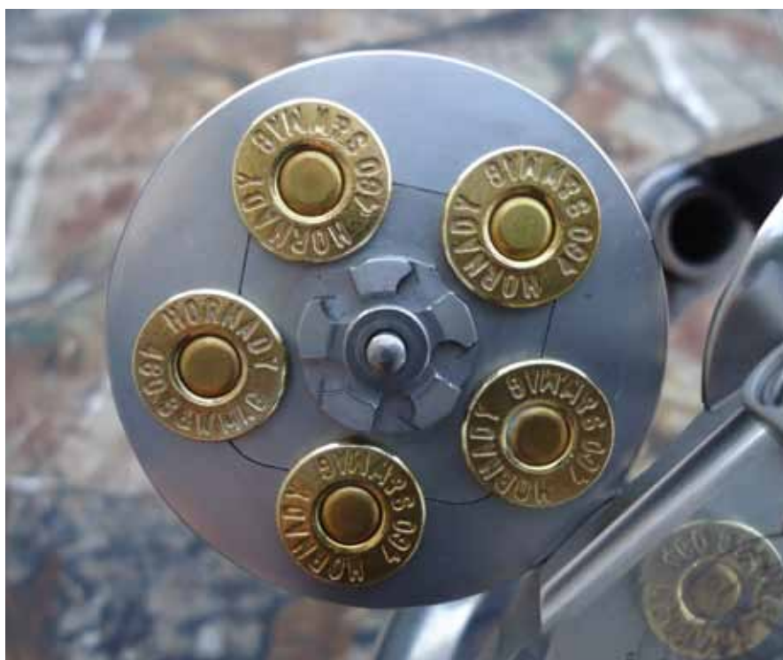
The thickness of the cylinder allows the containment of the massive pressure involved in shooting the .460 Magnum and five shots is enough to convince you of that.
