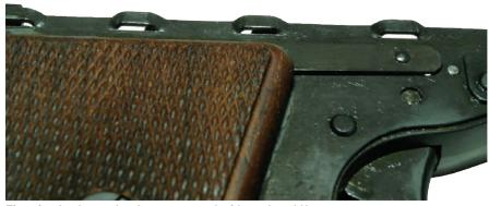
Five simple stamped-out areas on each side replaced the traditional machined guide rails on the receiver.
