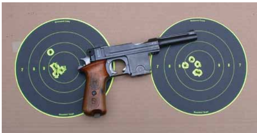
The M.1910/21 I test fired proved surprisingly accurate, as these groups fired at 50 feet prove.
