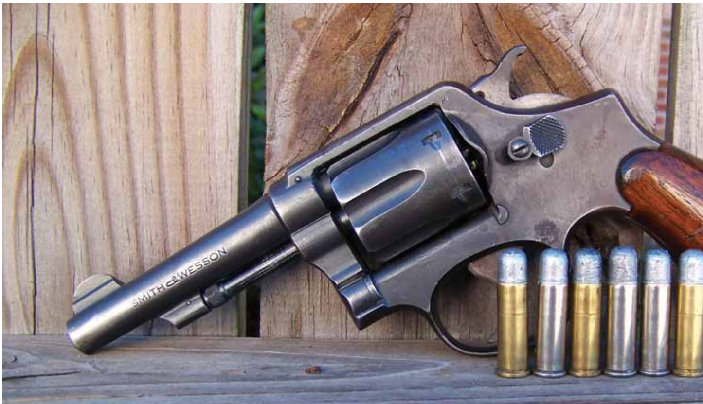
This is a Smith & Wesson 38 Special Victory Model. Note the 200-grain bullet handloads.
