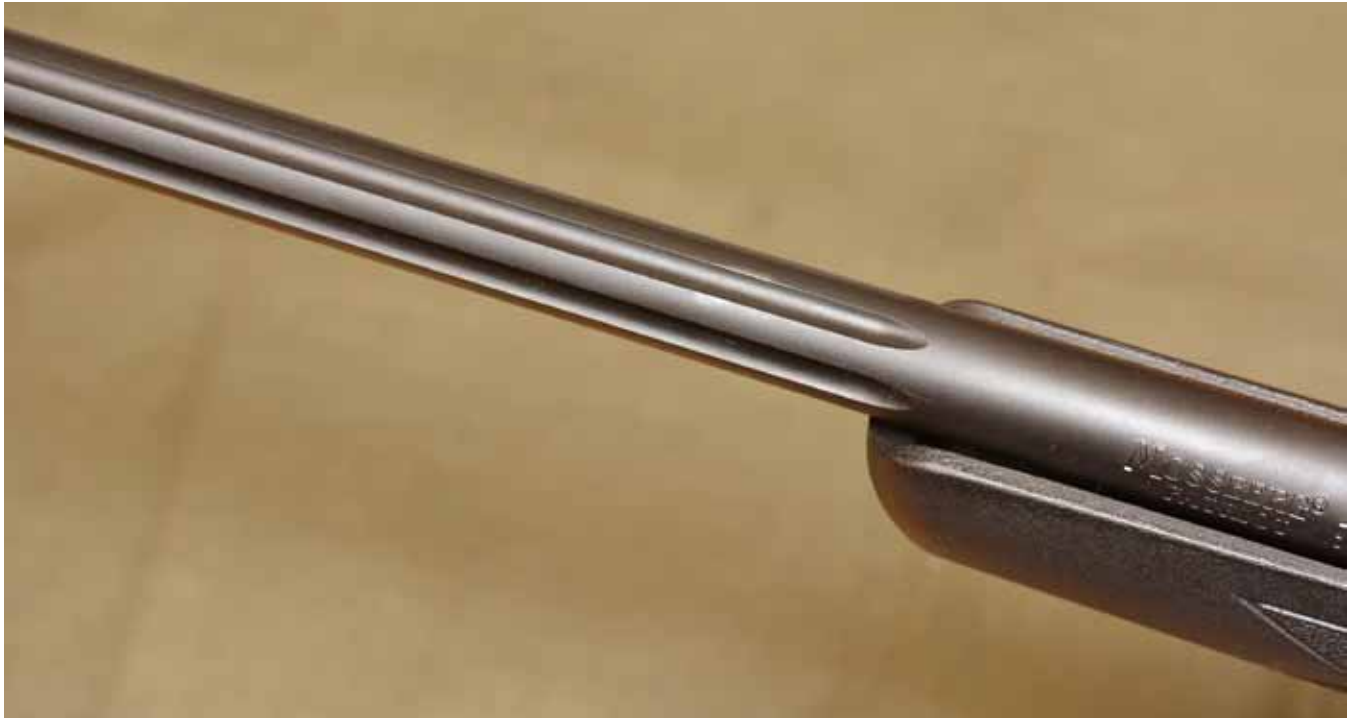
The barrel's fluting helps reduce weight to a small degree, but is largely cosmetic.
