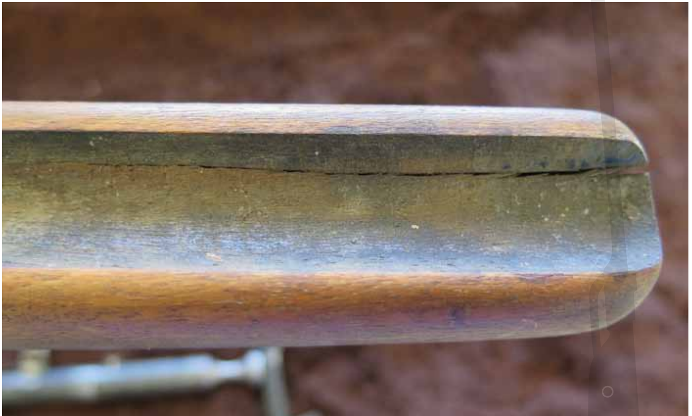
A cracked stock.
