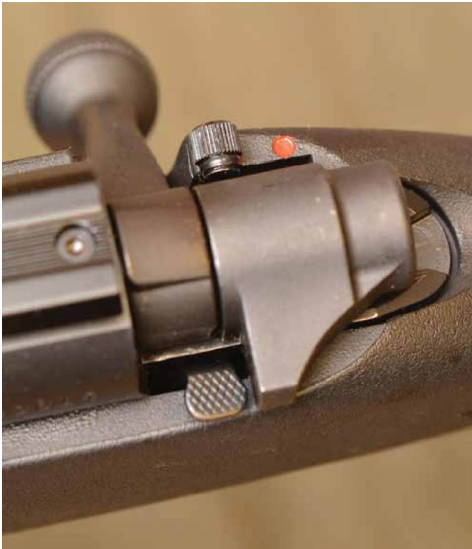
Top: The bolt body is fluted, and the two lug bolt head floats.
