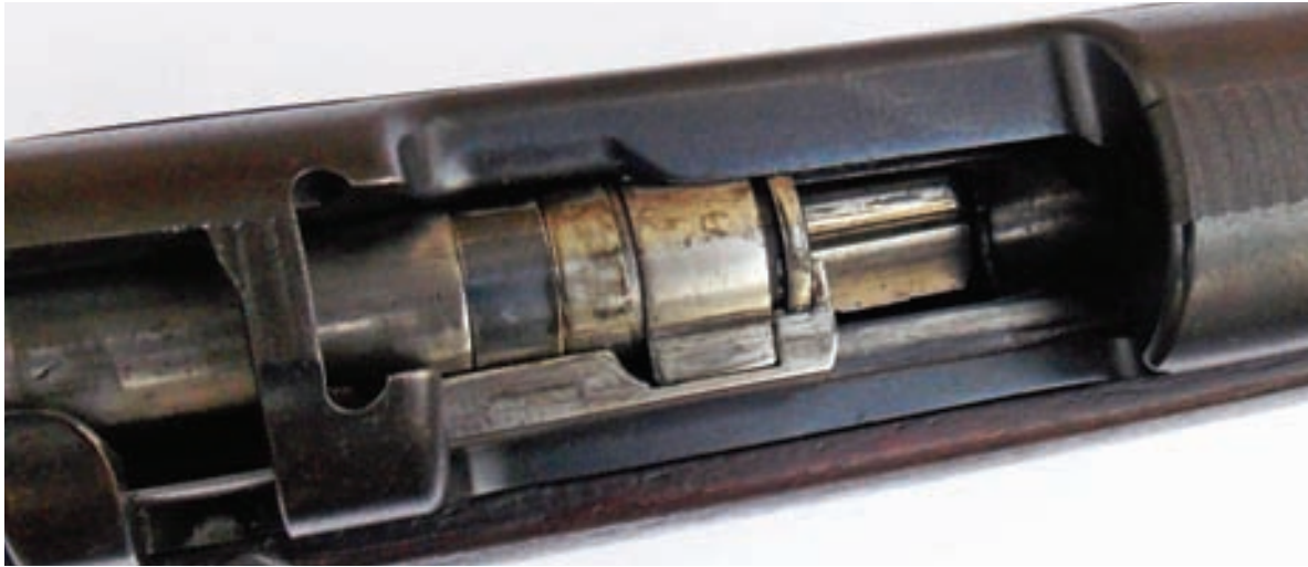
The bolt is Mauser-like and therefore has excellent feeding and extraction.
