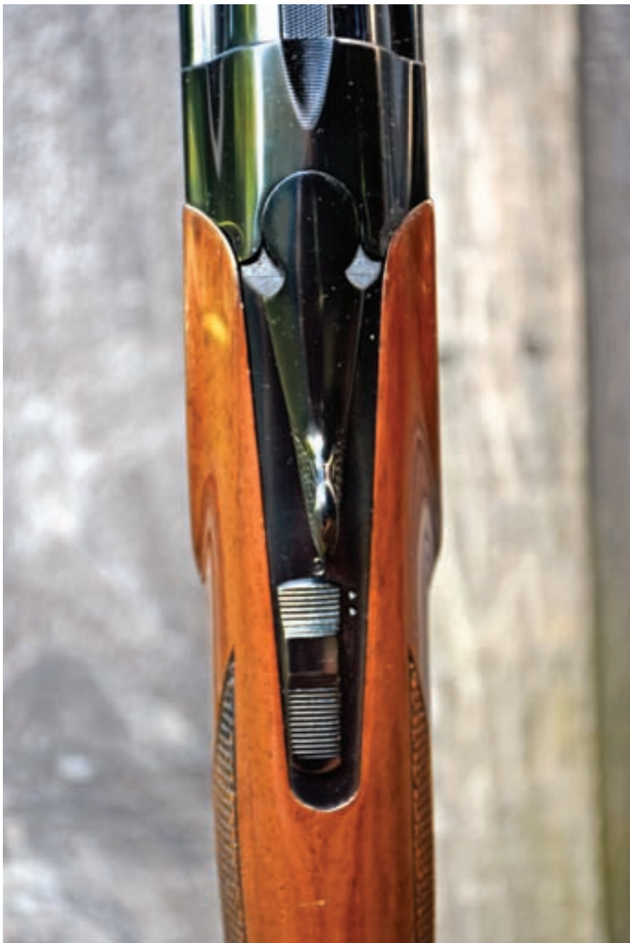
The safety also functions as a barrel selector.
