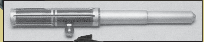
Left Top: Press-through fire selector for single and automatic fire. The grooved trigger and the patterned grip plates indicate a high-quality manufacturing. Left: The spring-loaded hook avoids accidentally withdrawing of the weapon when shooting from cover. Center: View of the bolt front with firing pin and extractor. Below: Bolt with dirt-protected telescope spring developed (and later patented) by Heinrich Vollmer.
