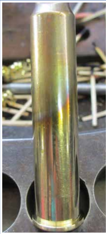
Left: An annealed case shows the characteristic coloration due to the heating of the brass. Above: The annealing station softens the shoulder/neck to ensure long case life.
