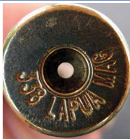
The case head after it has impacted the heading die (L Top) that carries the headstamp in reverse (Bottom - L).
