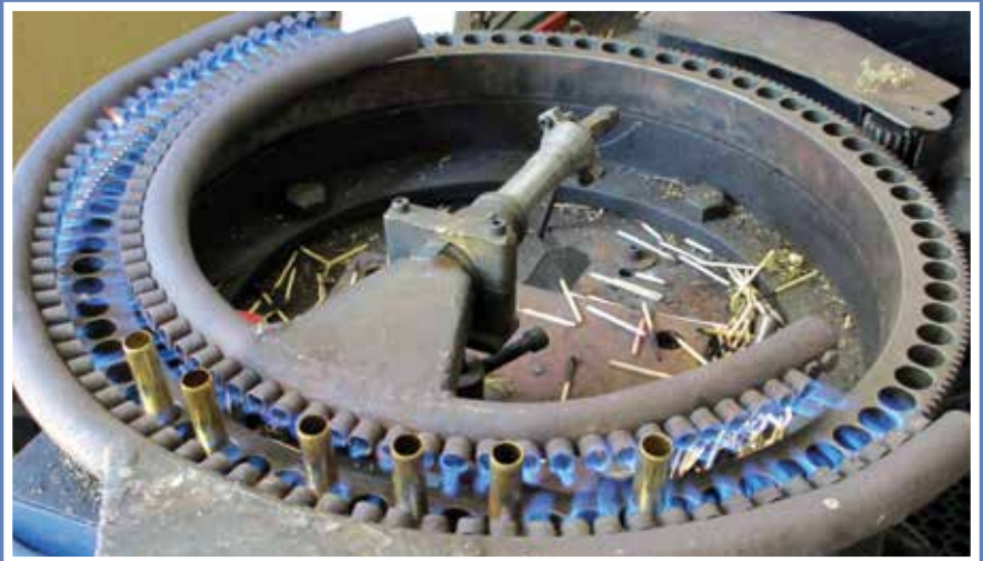
Left: An annealed case shows the characteristic coloration due to the heating of the brass. Above: The annealing station softens the shoulder/neck to ensure long case life.
