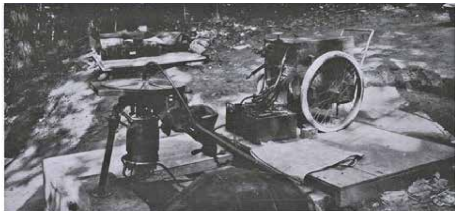
The Moore centrifugal machine gun, set up for test at the U. S. Bureau of Standards at the time of World War I. The grooved rotor was driven at high speed by a powerful electric motor. Steel ball bearings were fed into the center of rotor through the flexible pipe, and were delivered at a speed of about 1200 f.s. through the slot at left. The accuracy was extremely poor, but the inventor insisted that the gun would be useful in the trench warfare on the Western Front of 1918. The gun was not used.
