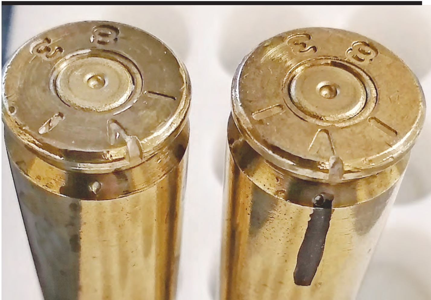
Notching rims is a permanent method of indexing cases, but it's not very visible.
