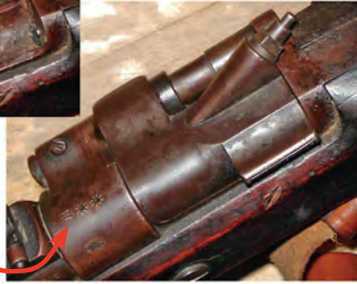
TOP: Conversion of an Enfield muzzleloader to accept early centrefire cartridges.
