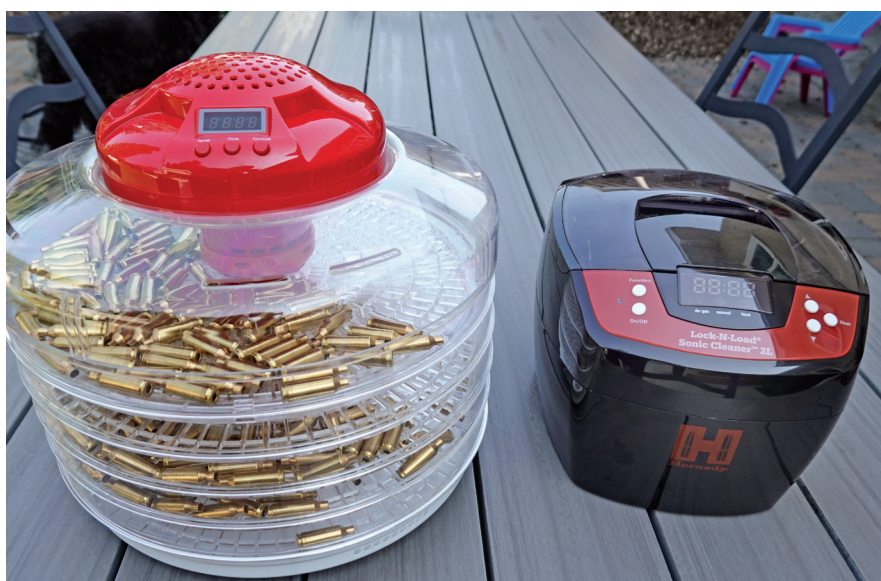
Hornady's ultrasonic cleaner and case dryer speed up the process of making several hundred cases shiny again.
